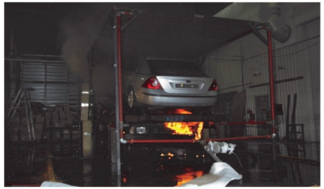
First Sprinkler Operated -13mins 6 secs. In total 3 sprinkler heads operate
