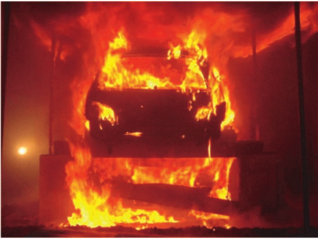
Car stacker burn test without sprinklers test after 10min 10 secs Photograph courtesy of BRE Global
